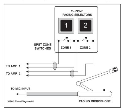
Fig. 18B - 2 - Zone Switching Panel
